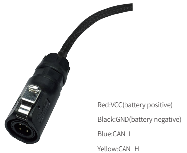
Figure 3.2 Schematic Diagram of Aviation Male Plug
